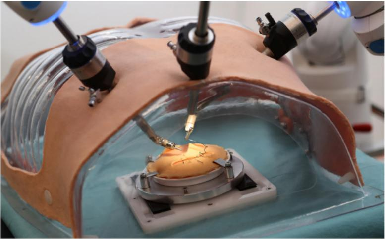
The research at the MIRO Innovation Lab has two main objectives: Firstly, the full dexterity of the surgeon's fingers and hands shall be projected into the patient to perform the manipulation tasks. Secondly, the information from inside the patient shall be acquired using sensors, be processed automatically and presented to the surgeon in an intuitive manner.
