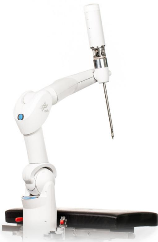
For highly precise manipulation tasks, the robot can be operated with position control. The specialisation of the versatile MIRO lightweight robot arm is provided by its instrumentation and application-specific software.
